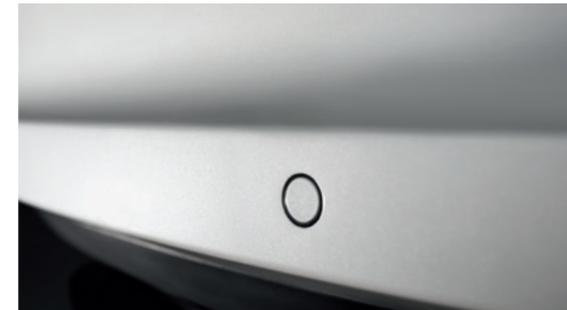
The XL1's rear is equipped with a Park Distance Control (PDC) system that warns you about obstacles at the rear of your car. As your car gets closer to an obstacle, the warning signal increases in frequency. Additionally, the display supports the driver by accurately showing the distance to obstacles.
