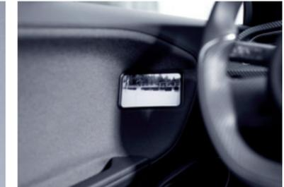
E-mirrors: Outside mirrors are replaced by small cameras on the wing doors that relay what is happening behind the car as well as smooth the air flow better than traditional mirrors. The images from the cameras are sent to display screens inside the vehicle without any time delay.
