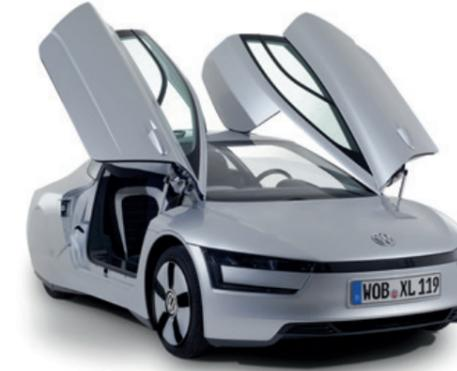
The wing doors extend far into the roof. They do not just swivel upward, but slightly forward as well – which creates an exceptionally large amount of entry and exit space.
