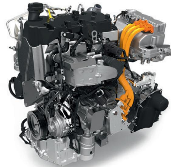
The lithium-ion battery that is integrated in the front section supplies the e-motor with energy. Operating at 220 V, the power electronics manage the flow of high voltage energy from and to the battery or e-motor and converts direct current to alternating current. The body electrical system of the XL1 is supplied with the necessary 12 V via a DC/DC converter and a small auxiliary battery.
