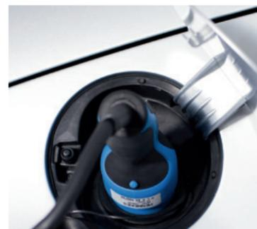
One of the most striking features of the Plug-in Hybrid car: the XL1 has two fuel filler flaps. Behind one is the conventional diesel tank, while the other covers the DC power connection. Ten liters of fuel and a battery with an energy content of 5.5 kWh enable a driving range of up to 500 km.
