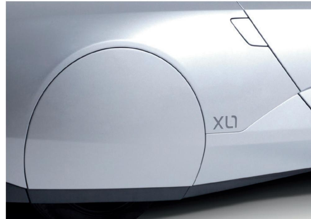
The rear wheel housing provides uniform air flow even around the rear section of the car, resulting in less turbulence and stalls.
