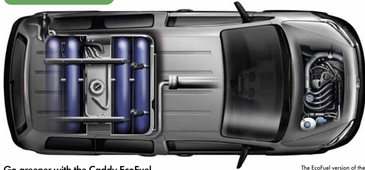
The EcoFuel version of the Caddy uses compressed natural gas (CNG) or biomethane, which both dramatically reduce emissions
