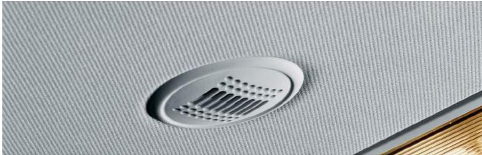
Optional Digital Voice Enhancement (DVE) provides voice amplification in the passenger compartment.
