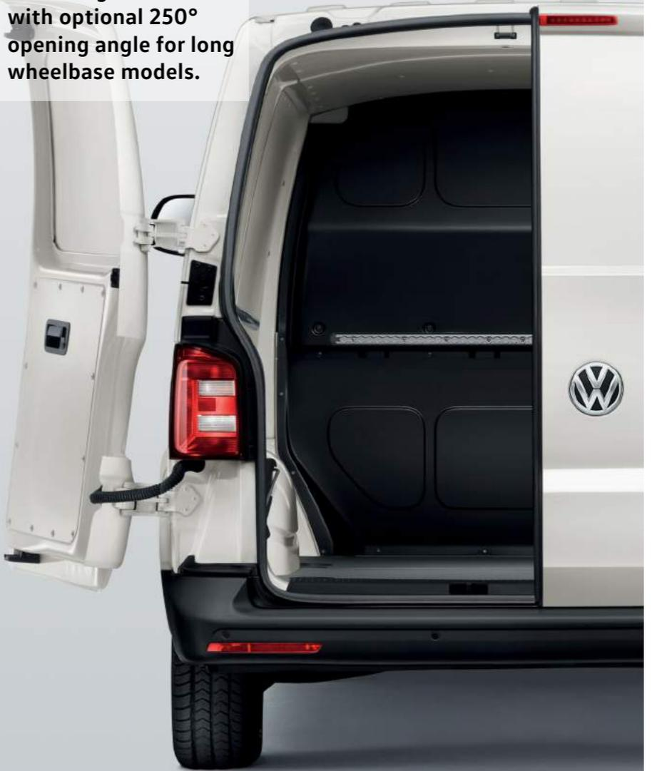
Image shown features rear wing doors without windows which are standard on panel van. Image also shows 250° opening angle hinges which are optional on long wheelbase models.
