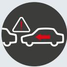
In town, City Safety is designed to prevent you from colliding with the car in front if it stops suddenly. This advanced IntelliSafe system works at speeds of up to 31 mph and senses if you're about to collide with another car, then, if necessary, applies the brakes.
