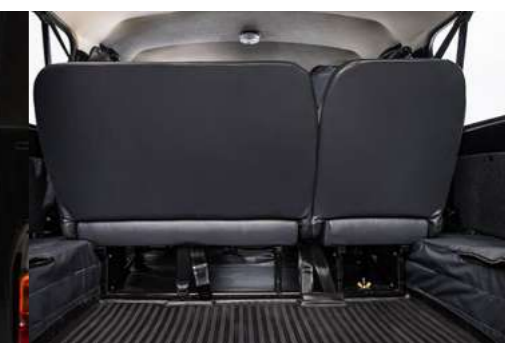
For transportation of large-size cargo and equipment the rear seats can be folded down 60/40 or turned into a bed by extending to 180°
