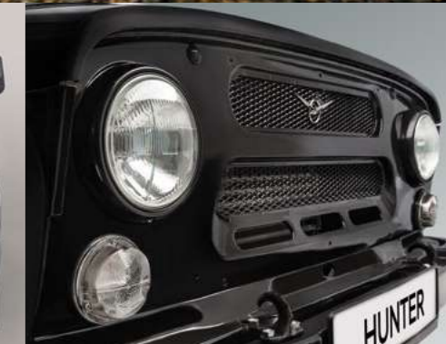
A metallic fine mesh grille protects the radiator from aggressive environment
