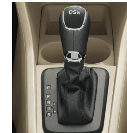
The **7-speed DSG** (Direct Shift Gearbox), supplied with the 1.4 TSI 125PS and 1.4 TDI CR 90PS engine, combines the advantages of mechanical and conventional automatic transmissions.
