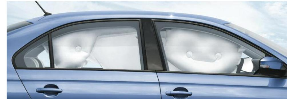
**Driver and passenger front, side and curtain airbags.** Should an impact occur, large-volume airbags activate in conjunction with the front seat belt pretensioners. This will anchor you in the middle of the seat and cushion you to reduce injury.
