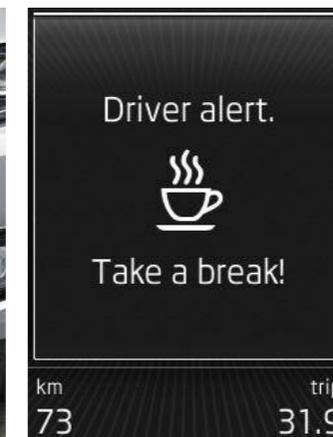
**Fatigue sensor.** Standard from SE is a Driver fatigue sensor. This monitors the movement of the driver through the steering wheel and if the driver begins to display signs of tiredness, the car will audibly alert the driver with a tone and show a break recommendation alert on the Maxi DOT.
