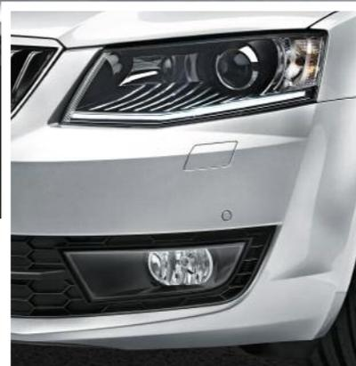
**Bi-Xenon headlights.** The optimal illumination of the Bi-Xenon headlights is enhanced by the AFS which changes the light setting depending of the car's speed and weather conditions. Bi-Xenon headlights provide 2.5 times the illumination of halogen headlights.
