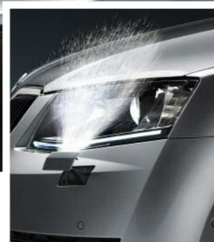
**Telescopic front headlight washers.** Standard on Scout, SE L, Laurin & Klement and vRS, optimise your front lights' range by keeping the front panels clean of dirt and debris.
