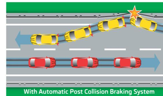
**Automatic Post Collision Braking System.** In the event of a crash, the Automatic Post Collision Braking System, standard on all Octavias, will be activated. This recognises when an impact has occurred and brakes the car to prevent it being uncontrollably propelled into oncoming traffic, reducing the risk of further crashes. The car will brake to 6mph and also activate the hazard and brake lights.
