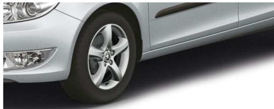
**Low rolling resistance tyres.** The Fabia GreenLine II has 15" 'Antares' alloys (6J x 15" 185/60 R15 84H) these lighter alloy wheels with low rolling resistance tyres have a higher prescribed air pressure to reduce friction.
