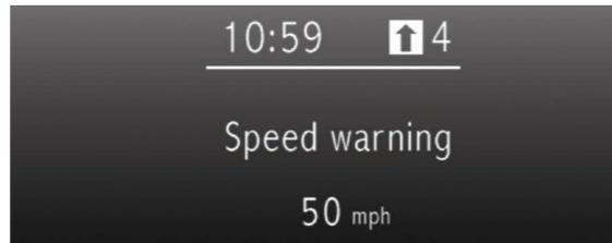
**Gear change recommendations.** The recommended gear feature on the trip computer or Maxi-dot display shows the driver whether the gear they are in is appropriate or whether they need to change up or down.
