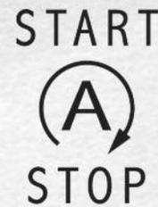
**Stop/start** lowers the Citigo combined fuel consumption by up to 9% percent. The standard 60PS has a combined fuel consumption of 62.8 mpg whilst the GreenTech achieves an impressive 68.9 mpg. During waiting times at red traffic lights or whilst sitting in traffic, the engine will switch off automatically, restarting as soon as the driver presses the clutch (or steps off the brake).
