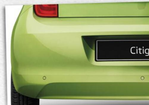
**Parking** the Citigo is easy due to its excellent manoeuvrability. There are three parking sensors integrated into the rear bumper, which check the car's distance from any obstacles. Optional on SE, Monte Carlo and SE L models.
