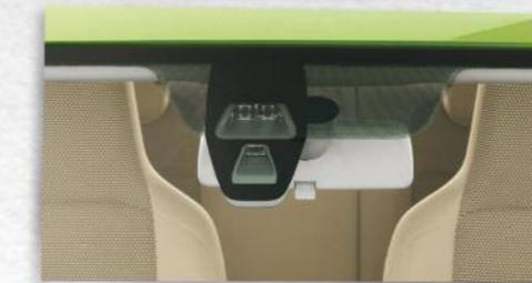
Citigo also features advanced technology - an optional 'City-safe' brake assist sensor that monitors the area in front of the vehicle, actively assisting braking at speeds below 19 mph when there is danger of a collision. Please note that it is the driver's responsibility to be in control of the vehicle at all times.
