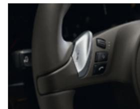
PDK gearshift switches on multifunction steering wheel
