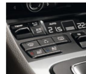
Seat heating, seat ventilation, two-zone automatic climate control
