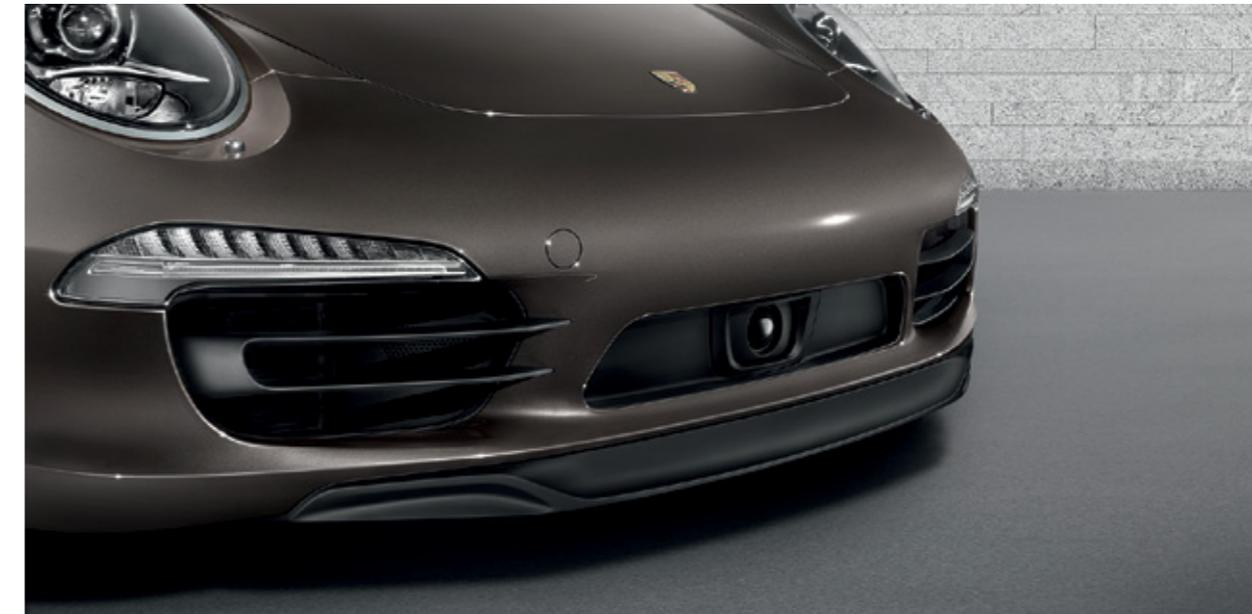
Radar sensor of adaptive cruise control
