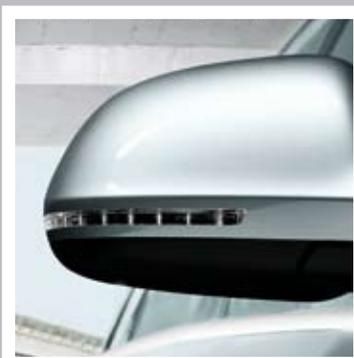
Exterior mirrors – electrically operated and heated
