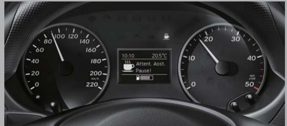
ATTENTION ASSIST, a standard feature, is able to detect the typical signs of fatigue based on numerous parameters and so warn the driver.
