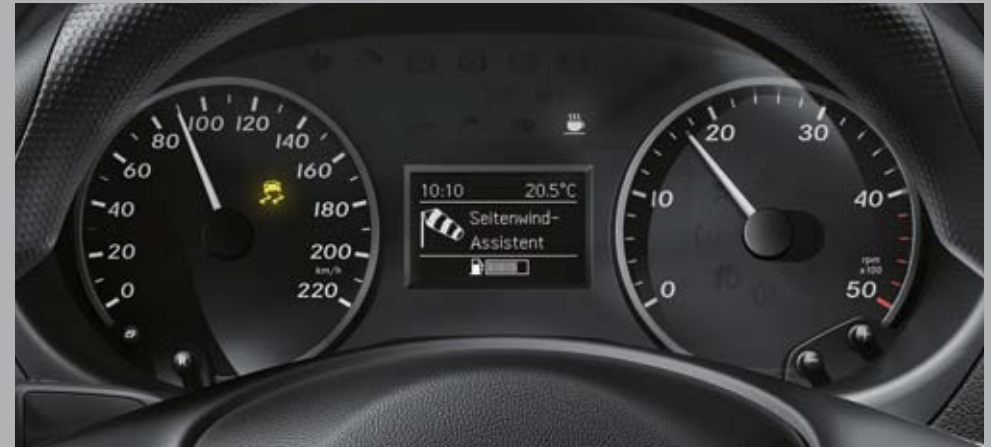
The standard-fit Crosswind Assist helps to prevent lateral drift of the vehicle due to gusting crosswinds.
