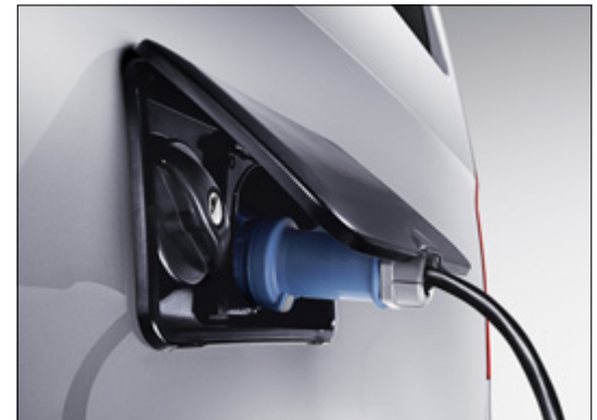
External connections for power and fresh water
