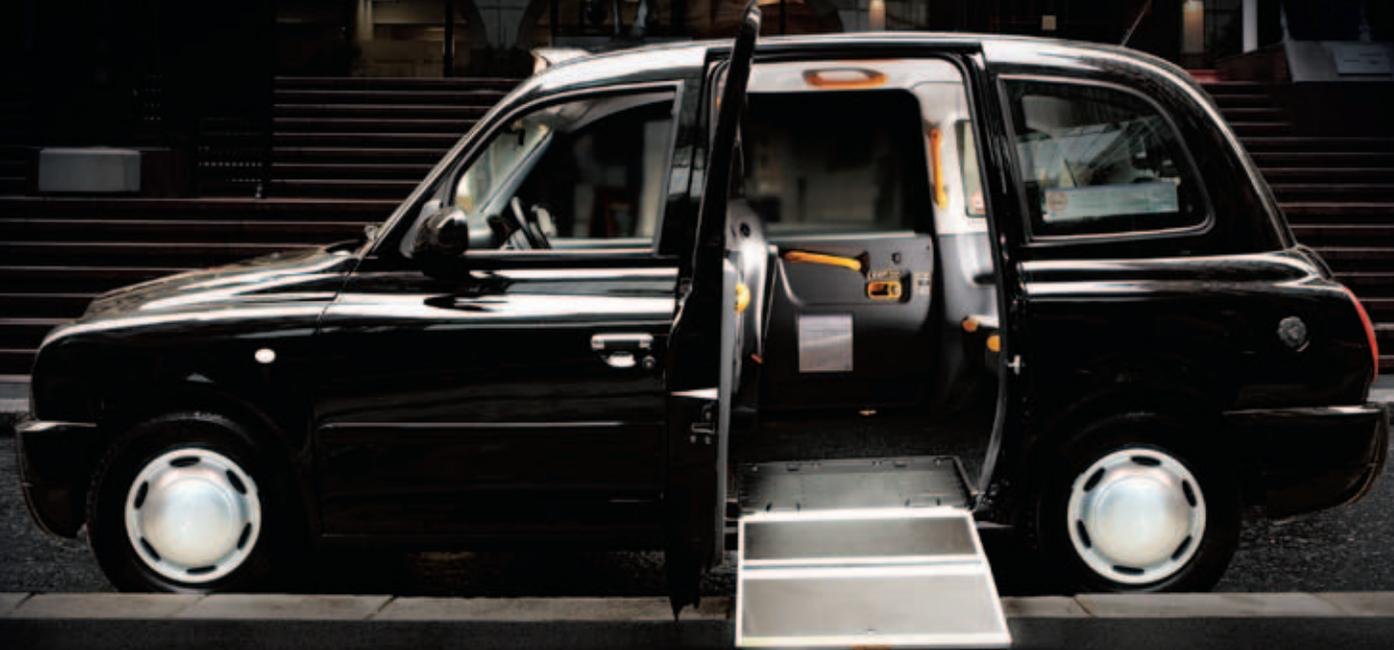
Integral ramps allow easy access, with a securing mechanism for wheelchair users providing stability during the journey.
