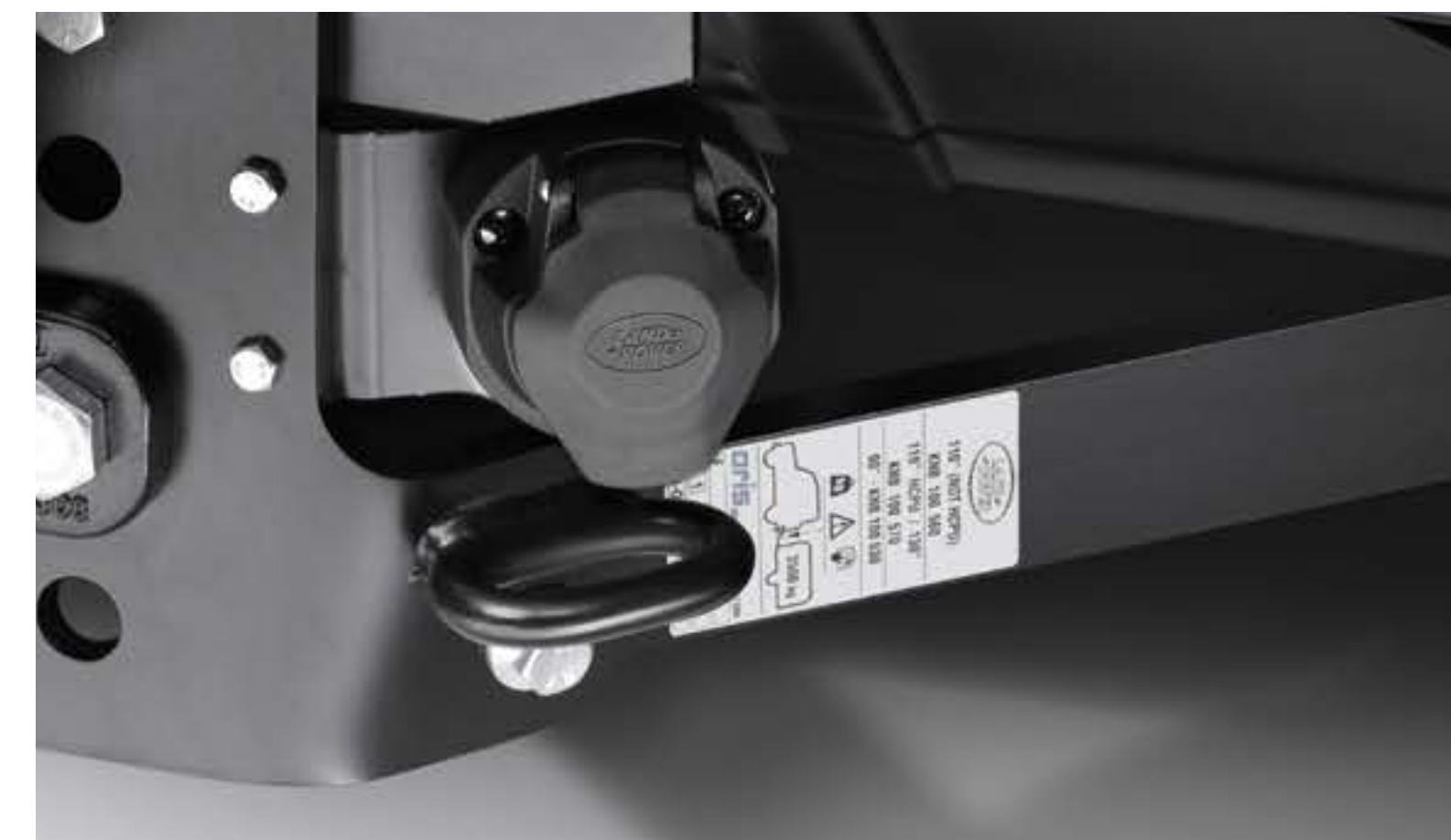
13 Pin Towing Electrics** LR005919 European style towing electrics, capable of supplying all trailer rear lighting and interior equipment power, including fridge feed and battery charging.
