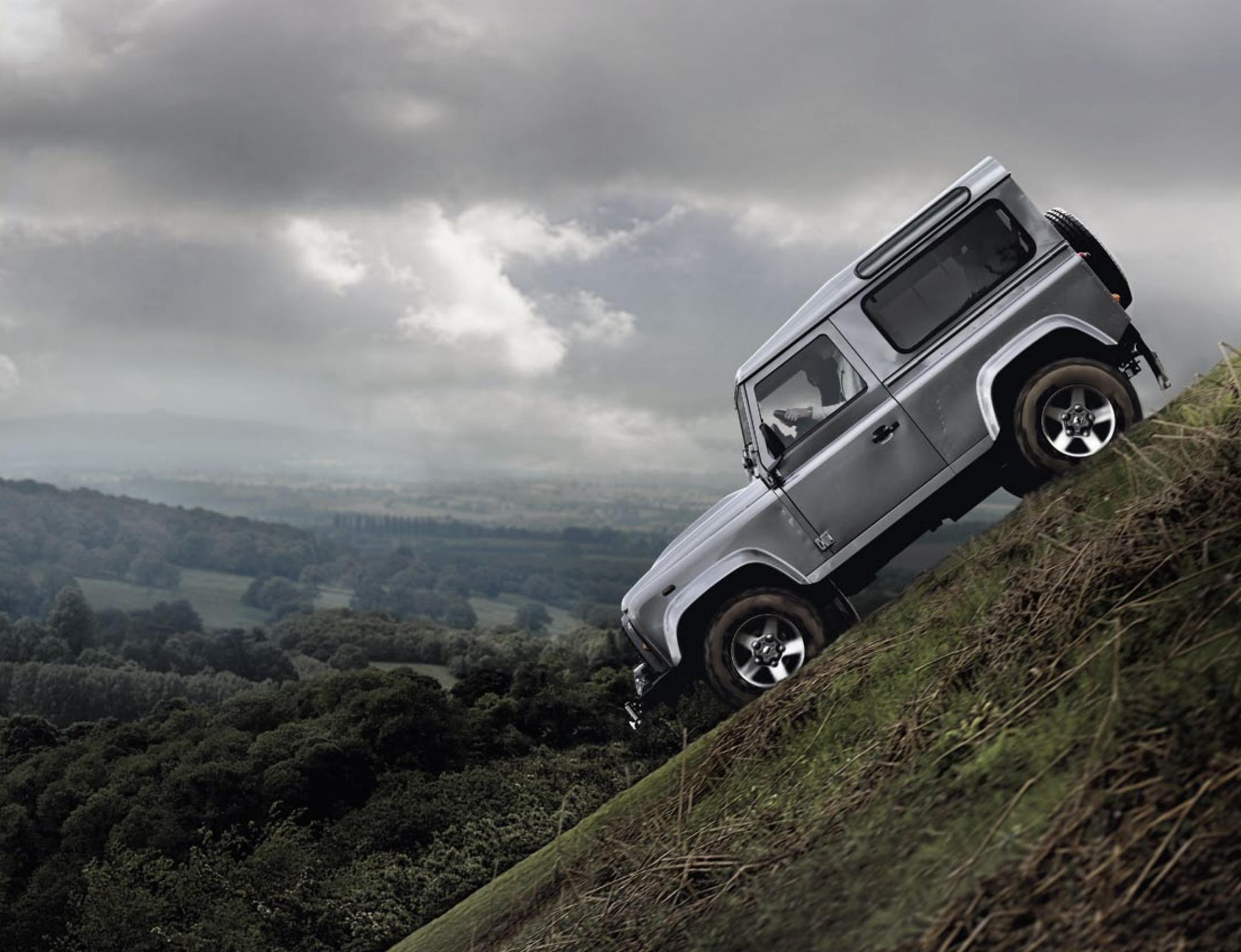
Unlike many of its competitors, Defender has permanent four-wheel drive with the centre differential distributing torque evenly between front and rear axles to give optimum performance on-road and off-road. What's more, the centre differential can be locked to help minimise wheel spin and maximise traction on slippery surfaces. And for even more grip and control off-road (not to mention on-road as well) Defender is available with an optional ABS system featuring traction control.
