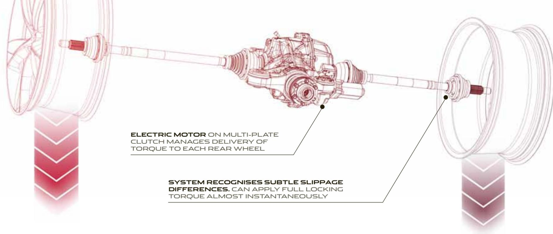
**ELECTRIC MOTOR ON MULTI-PLATE CLUTCH MANAGES DELIVERY OF TORQUE TO EACH REAR WHEEL**
