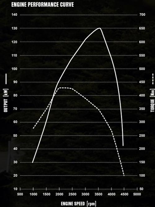
The Isuzu D-MAX range is powered by a highly refined 3-litre turbo diesel common rail engine which offers superior fuel efficiency thanks to low friction, fuel injection optimisation and a large front-mounted intercooler.
