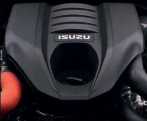
Isuzu 4JJ1-TC Hi-Power turbo diesel engine offers a maximum torque output of 430Nm and 130kW of power
