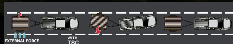
Designed to recognise early signs of dangerous trailer sway, Trailer Sway Control (TSC) automatically applies the brake on individual wheels, as well as reducing engine torque, to bring the trailer safely back under control
