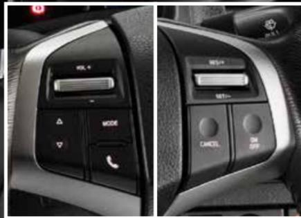
All LS-models<sup>^</sup> are equipped with steering wheel cruise, audio and Bluetooth<sup>®</sup> function controls
