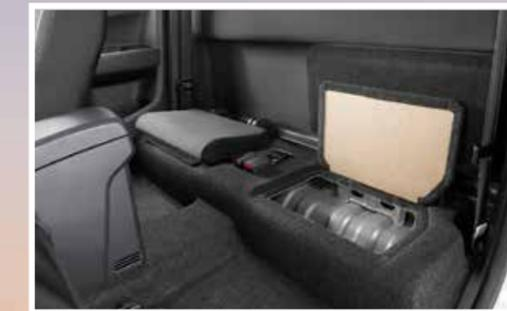
Fold down rear seats in Space Cab with storage compartments
