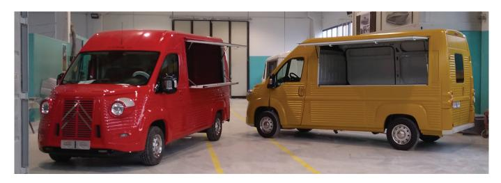
Swinging side openings available in three versions: single hatch (with or without flap) or double.
