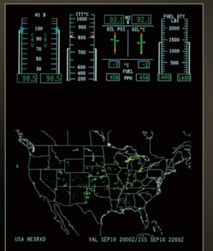
Broadcast Graphical Weather – ground-based weather data ahead of the flight route
