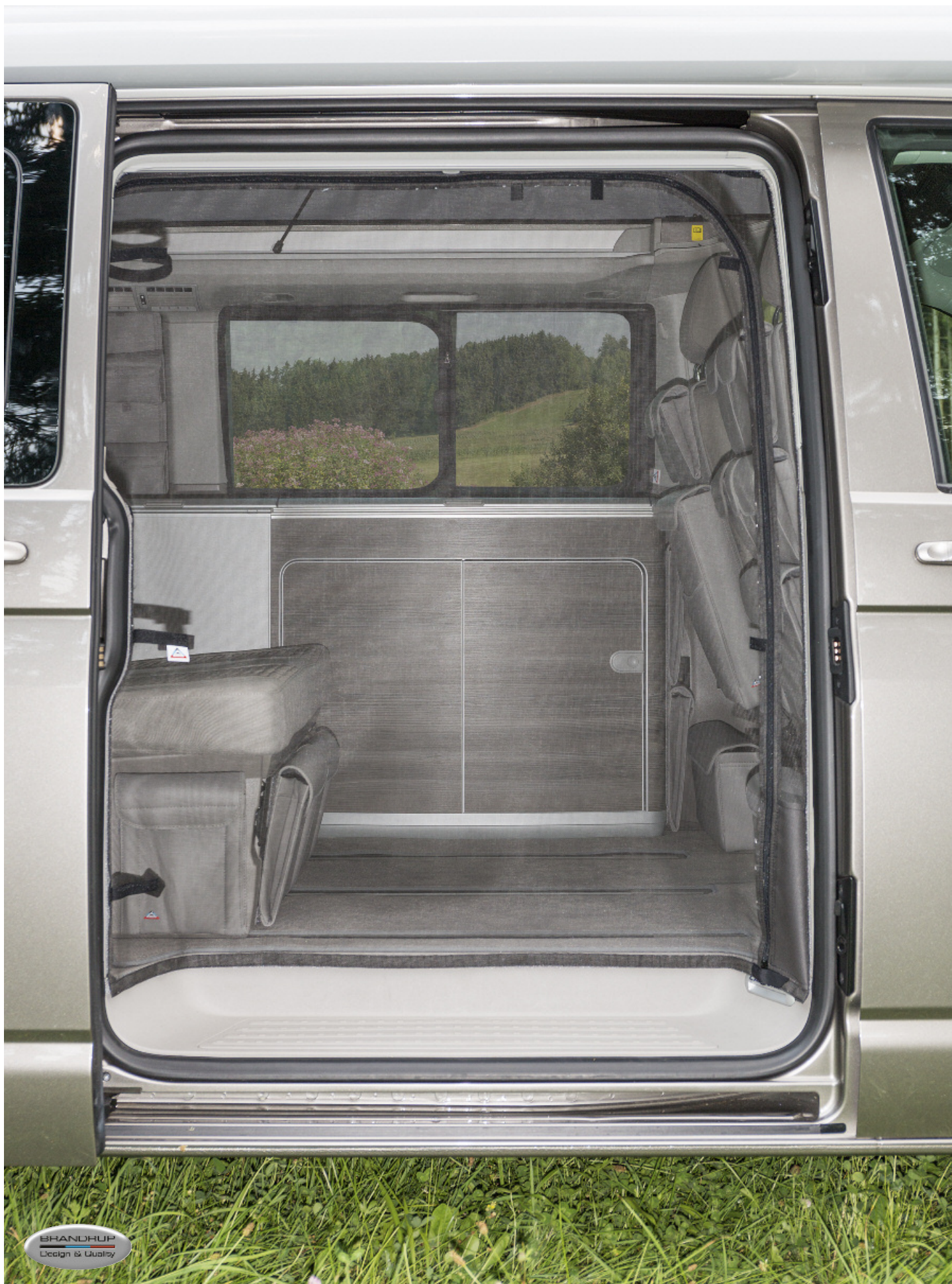
The FLYOUT has an arched zipper which can be operated from every position of the bench.
