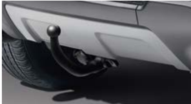
Detachable Tow Bar VPLVT0166 European style towing electrics, capable of supplying all trailer rear lighting and interior equipment power. 12N/12S Type Towing Electrics Adapter** (shown above) VPLHT0060 12N Moulded Adapter** VPLVT0064
