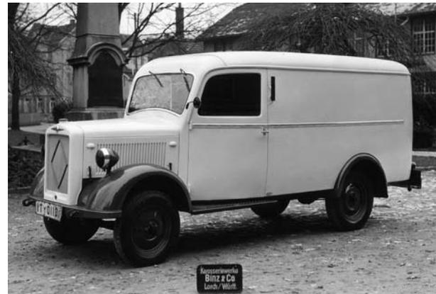
workers extend the chassis frame, I can take care of the body and the wider door. That's the perfect job for me." The metalworkers then extended the frame. And the wheelwright workshop staff got to work. The body was cut and pulled apart in the door area and jointed 30 centimetres in between. Two wide doors were manufactured, covered in sheet metal and painted.
