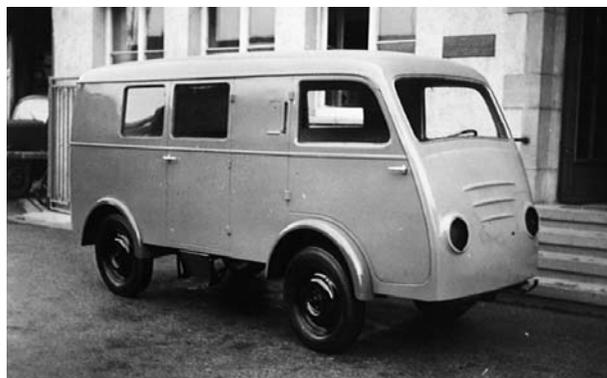
instead of a separate box body. As a result, BINZ created the first prototypes of a functional, plain and simple small box-body truck in 1949. The outer features of the prototypes differed from the Vischer cars by their one-piece windscreen and the three cross beads on the front of the vehicle.
