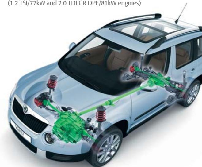
**Škoda Yeti with a 4-wheel drive and a 4th generation Haldex clutch**
