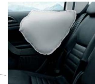
The **rear side airbags**, which are activated by a side impact, protect the pelvis and chest of passengers on the rear side seats.
