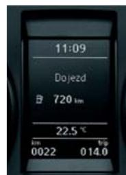
The multifunctional **Maxi DOT** display is located in the centre of the instrument panel.
