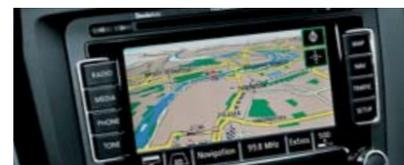
The **Columbus navigation system** offers, amongst others, off-road navigation. This feature enables you to record and save a route taken by the vehicle off the digitised road network, for example on unpaved roads.
