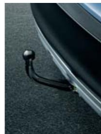
A **towing device** for a trailer of up to 1,800kg.
