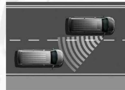
**Lane Change Assist<sup>1,2</sup>** has radar sensors to help monitor traffic. When you change lanes, the system warns you via flashing lights in the exterior mirrors if another vehicle is identified within the blind spot.
