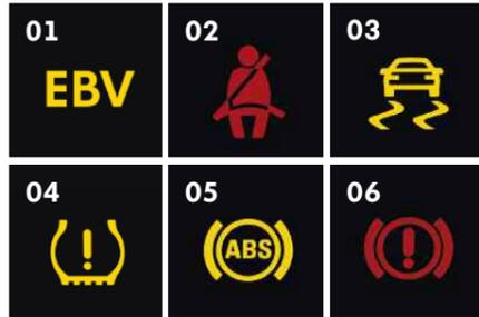
**01** When the vehicle weight is transferred to the front wheels during braking, the **Electronic Brakeforce Distribution (EBD/EBV)** prevents lockup of the rear wheels, which are under less load. This helps your vehicle brake safely in a straight line.
