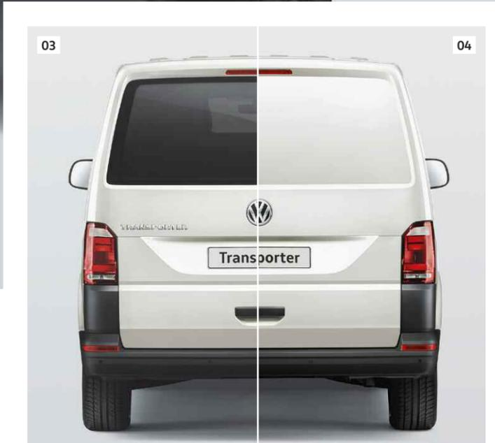
**01** Main image features rear wing doors without windows which are standard on panel van, while optional on kombi. Image also shows optional 250° opening angle hinges.
