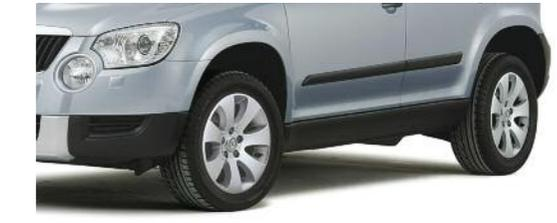
**Aerodynamics.** One of the simplest ways to improve fuel efficiency and reduce emissions, is to create a more aerodynamic vehicle. The Yeti GreenLine II has slightly lowered suspension to facilitate better airflow.
