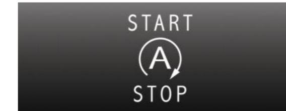
**Stop/start System.** This innovative system turns off the engine when it is not needed, for example when the driver is stopped at traffic lights or in heavy traffic.
