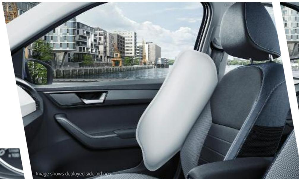
Image shows deployed side airbags
