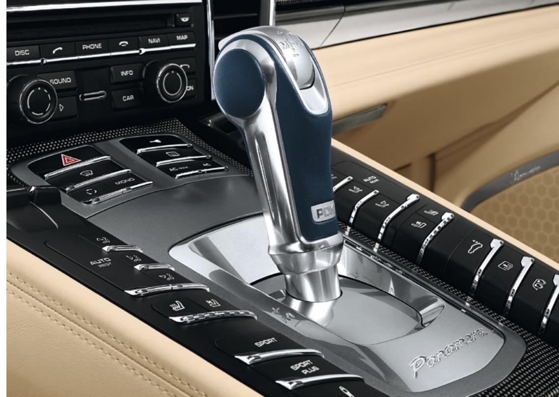
PDK gear selector in aluminium
