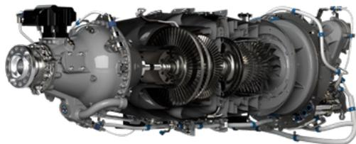
*With Pratt & Whitney's PT6E-67XP engine, the PC-12 horsepower-to-weight ratio is comparable to a P-51 Mustang fighter.*
