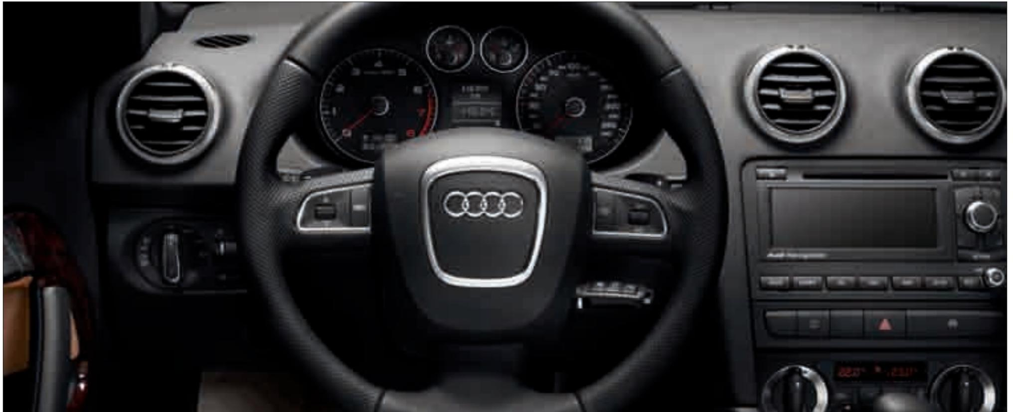
3-spoke multi-function steering wheel with gear-change controls
