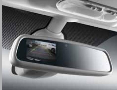
○ The **reversing camera** with display in the rearview mirror provides a view of the area to the rear, assisting the driver in tight parking and manoeuvring situations. Dynamic guidelines are displayed as an additional aid.
