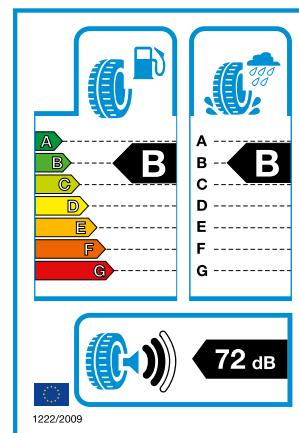
Specifications acc. to EU Directive 1222/2009. Tyre labelling provides information about three key factors relating to tyre performance:
