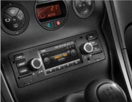
○ The **navigation system**<sup>1</sup> incl. DAB+ radio and integrated touchscreen display is easy to use. With Bluetooth®, USB port, AUX interface and micro SD card reader.
