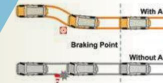
Anti-lock Braking System (ABS)
