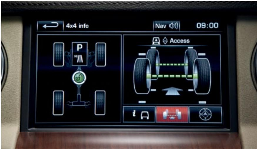
**AIR SUSPENSION.** Four-corner independent air suspension features variable ride height and electronic cross-linking for a constant level ride height irrespective of load distribution. Ride height can be raised up to 125mm to clear obstacles or lowered by 50mm for easy access and loading.
