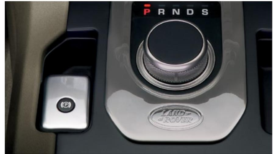
**ELECTRIC PARKING BRAKE (EPB).** A switch next to the eight-speed Drive Select is designed to electrically apply and release the parking brakes on the rear wheels. A simple pull of the lever applies the brake manually and a press releases it. The parking brake will also release automatically upon drive away.
