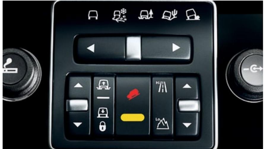
**TERRAIN RESPONSE® SYSTEM.** Optimises the vehicle set-up for virtually all on-road or off-road driving situations, with five different settings to suit different terrains such as Grass/Gravel/Snow, Sand, Mud and Ruts and Rock Crawl.
