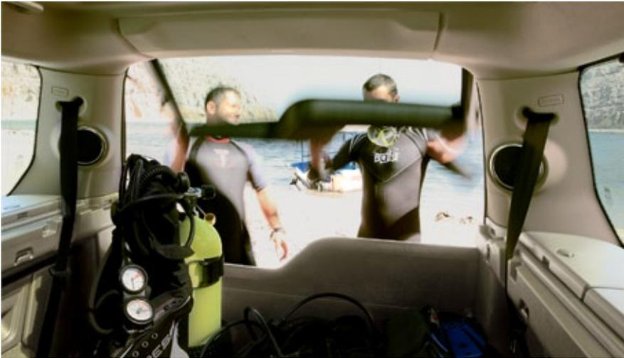
**SPLIT TAILGATE.** Make light work of difficult loads with Discovery 4's two-piece, asymmetric tailgate design. Both upper and lower tailgates are made from resilient lightweight aluminium. The tailgate gives impressive access to the rear of the vehicle and comes into its own when loading large, bulky or heavy objects. The asymmetric portion of the lower tailgate provides a reduced reach-in distance when open and a lower load height when closed.
