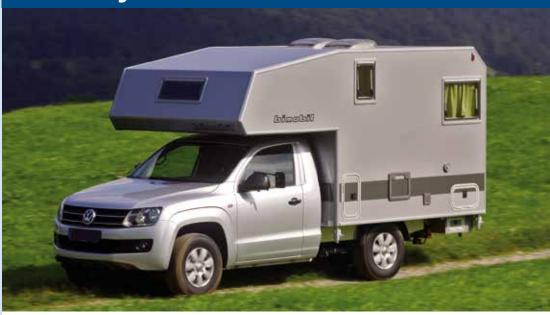
The VW Amarok Single Cab is the ideal two person vehicle, providing spacious accommodation in the Husky 270 habitation cabin. Two engine sizes are available, a fuel-saving 90 kW (122 Hp) and a powerful 132kW (180 Hp) version.
