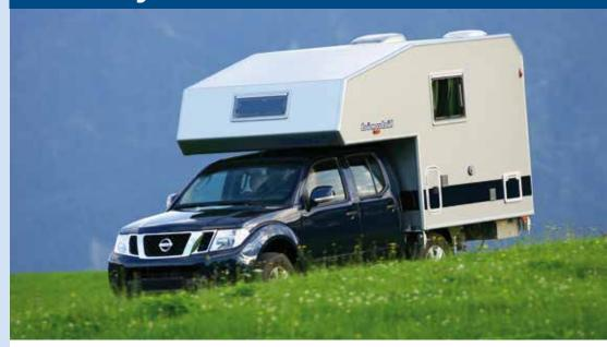
The Husky 230 is a fully-fledged motorhome built onto a Nissan Navara double-cab pickup. The Nissan seats four to five people comfortably, so when fitted with the Bimobil interchangeable demounting system, can be used at home as a five-seater car or on holiday as a family run-around, while leaving the cabin demounted at the overnight site.
