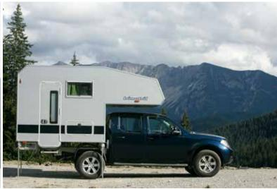
The original vehicle load-bed is removed from the pickup, but can be fitted with a demountable frame, so that the motorhome can be converted back to a fully-fledged pickup at any time. A small crane (available as an accessory) can be used to facilitate mounting and demounting the load-bed. Hard or soft tops fitted to the load-bed do not normally have to be removed when mounting or demounting.
