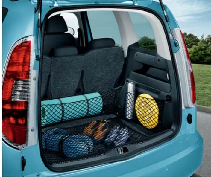
Even with the seats in their base positions and with five passengers in the vehicle, an exceptional **luggage compartment** is at your disposal. Its capacity is, depending on the position of the rear seats and backrests, between **480 and 560 litres**. In addition, we offer you various accessories, which increase the practicality of the luggage compartment and help you keep the car tidy. For example, the **set of nets** prevents movement of, and possible damage to, the transported luggage.
