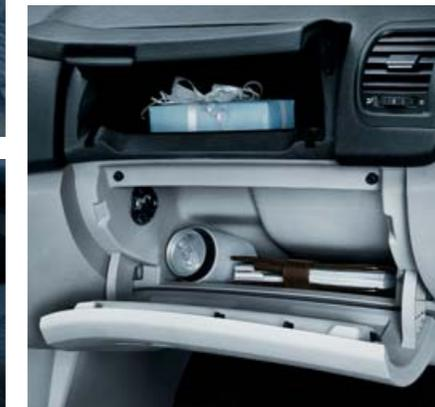
The **storage compartments in the dashboard** are available in two versions, either open or closed. The lower compartment may be illuminated and, in combination with the Climatronic air conditioning, cooled.
