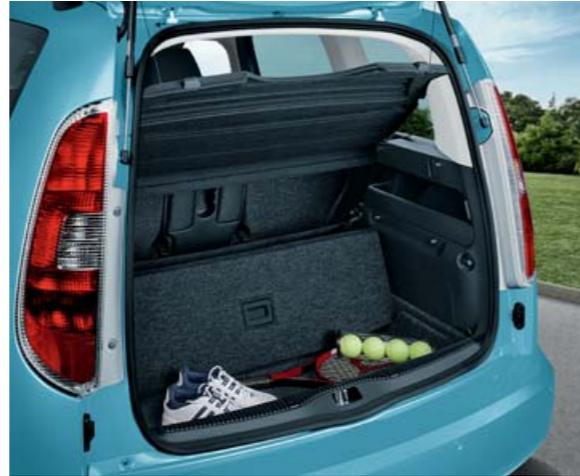
The **mid-level luggage compartment floor** provides a suitable storage place to keep things that you don't want to unload every day. In addition, it places the bottom of the luggage compartment on the level of the loading edge, facilitating easier luggage handling.
