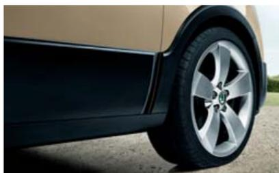
**Plastic covers** on the bumpers, sills and lower parts of the doors emphasise the car's uniqueness, along with **alloy wheels** especially developed for the Scout, available in the same design in two different sizes: the 6.5J x 16" **Arktos** (see photo) and the 7.0J x 17" **Kentaur**.
