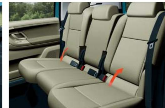
You can **shift** the **rear side seats** 80 mm forward and 70 mm backward from their base positions. The **backrests** of the seats can be **positioned** as needed.
