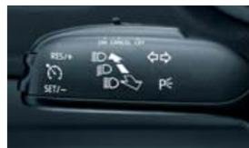
In addition to maintaining the preselected speed, **cruise control** enables you to increase or reduce speed without using the pedals. This function is controlled by the button on the side of the cruise control.
