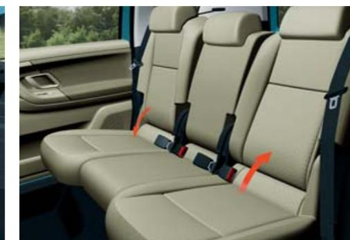
You can **shift** the **rear side seats** 80 mm forward and 70 mm backward from their base positions. The **backrests** of the seats can be **positioned** as needed.
