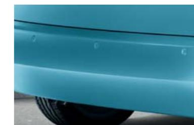
When manoeuvring the vehicle in a tight space, you will appreciate the **parking sensors**, which monitor the distance of the rear bumper from a potential barrier.
