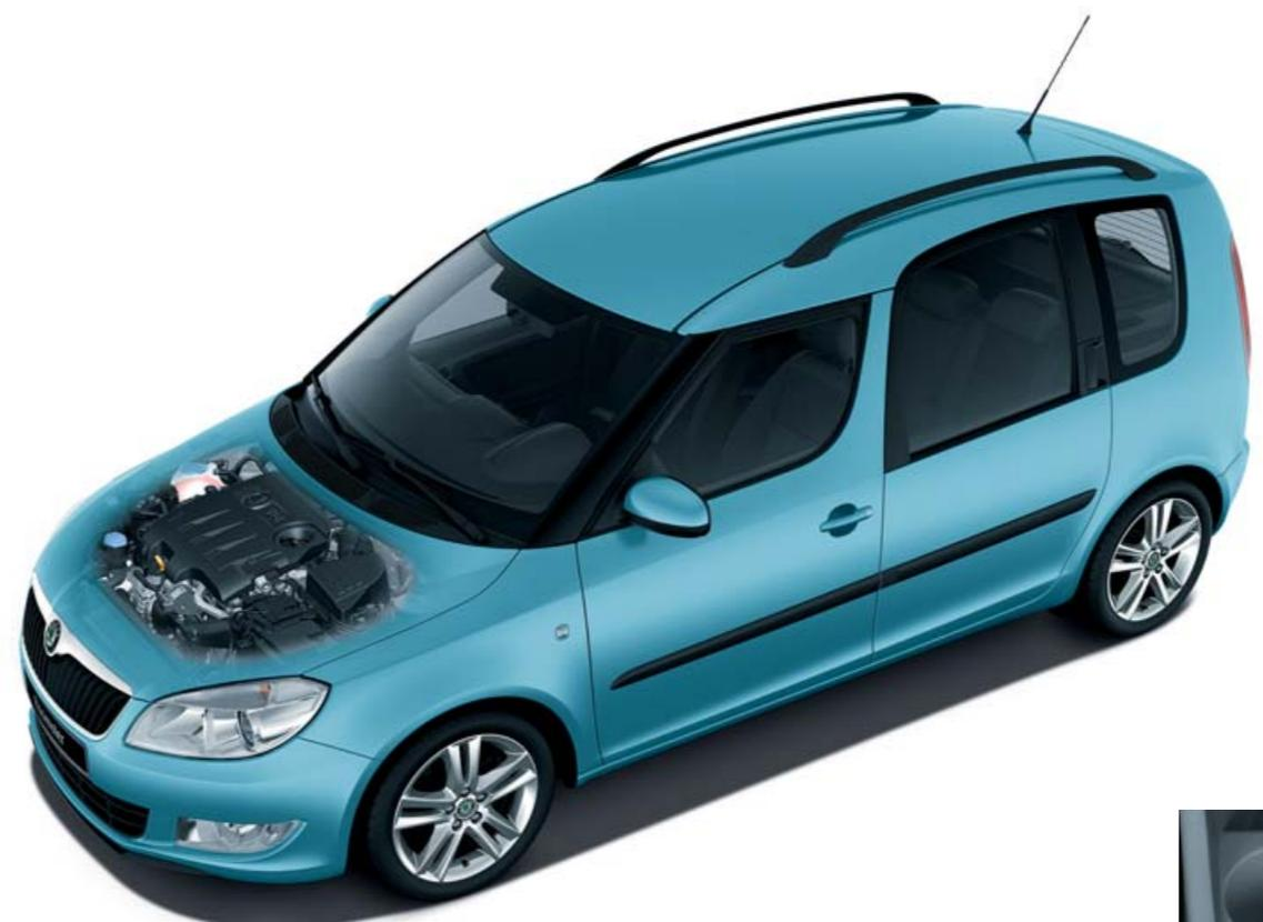
The highest performance diesel engine developed for the new Roomster is the **1.6 TDI CR DPF/77kW** turbocharged 4-cylinder engine.
