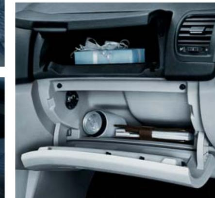
The **storage compartments in the dashboard** are available in two versions, either open or closed. The lower compartment may be illuminated and, in combination with the Climatronic air conditioning, cooled.
