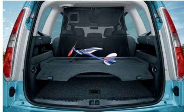
The **dividing net**, usually fixed behind the rear seats, separates the cabin from the luggage compartment. The **2-position luggage compartment cover** allows, when fixed in the lower position, the transport of objects that would otherwise impede the driver's view.
