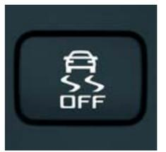
You may order additional features, such as **TPM** (Tyre Pressure Monitoring) and **start-up assistant**, supplementing the **ESP** (Electronic Stability Programme), which always includes **ASR** (Anti-Slip Regulation; deactivation button shown on the photo).
