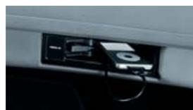
The **MDI** (Mobile Device Interface) enables (by means of interconnecting cables with terminals for the iPod, Aux-in or USB, available from Škoda Genuine Accessories) control of a connected external device through the radio or navigation system.
