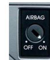
If you wish to place the child seat on the front passenger seat, you'll need to equip your car with the optional **deactivation of a passenger airbag**. Once installed, you can turn off the airbag with a key.
